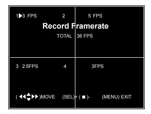
The total number of photos taken per second is divided among the cameras. The total frame rate of all the cameras in use is set to 60fps (frames per second). The higher settings produce better images, but use up more hard drive space.
